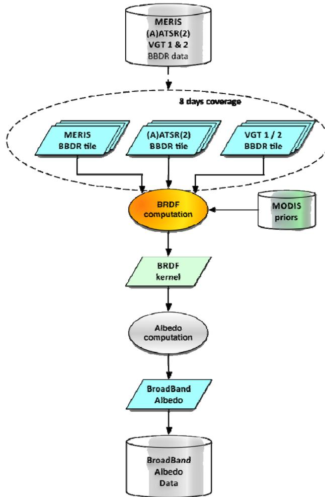
Figure 4-3: Generation of multi-sensor 8 day and monthly composites from BBDR inputs
